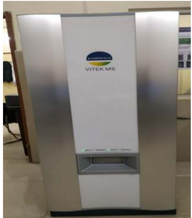
Matrix Assisted Laser Desorption Ionization - Time of Flight (MALDI- TOF) : (For Automated Bacterial/Fungal Identification)
